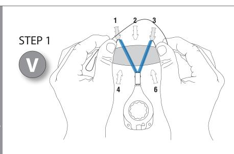
Using both hands, grasp the tension line near the front of the tension controller and with the first movement form the letter **V** by going around the tabs of anchors #1 and #3.
