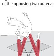
Holding the tension line with one hand, guide line over the final anchor tab opposite the tension controller, completing the letter **W**. Gently pull back on the tension controller to remove any slack in the line.
