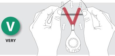
Using both hands, grasp the tension line near the front of the tension controller and with the first movement form the letter **V** by going around the tabs of the top two outer anchors.
