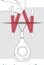
Holding the tension line with one hand, guide line over the final anchor tab opposite the tension controller, completing the letter **W**. Gently pull back on the tension controller to remove any slack in the line.
