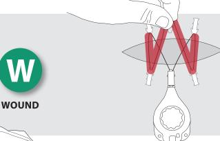
Holding the tension line with one hand, guide line over the final anchor tab opposite the tension controller, completing the letter **W**. Gently pull back on the tension controller to remove any slack in the line.
