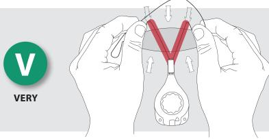
Using both hands, grasp the tension line near the front of the tension controller and with the first movement form the letter **V** by going around the tabs of the top two outer anchors.
